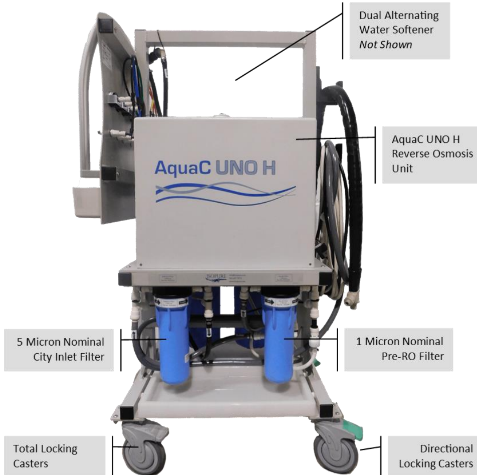
Figure 3. Prefilter Diagram
